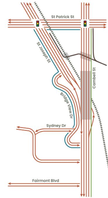
This alternative would retain the existing street configuration in the study area. A trail connection would be added along the existing drainage way that goes underneath Cambell Street and the railroad, with connections up to St. Joseph Street and Creek Drive on the west and east ends, respectively. Sidewalks would also be added to St. Joseph Street, Bridge View Drive, and Cambell Street.
