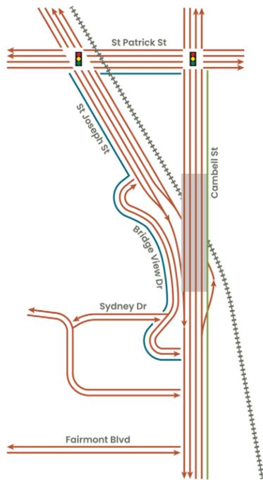
This alternative would retain the existing street configuration largely as is, with the Cambell Street railroad crossing changed from grade-separated to at-grade. Sidewalks would be added along St. Joseph Street, Bridge View Drive, and Cambell Street.
