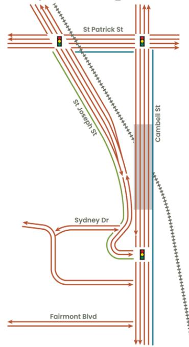
This alternative would eliminate the existing on/off-ramps that connect St. Joseph Street and Cambell Street. St. Joseph Street and Bridge View Drive would be merged into a continuous alignment, and a new traffic signal would be added to the intersection of Cambell Street and St. Joseph Street. Sidewalks would be added to Cambell Street and St. Joseph Street/Bridge View Drive.
