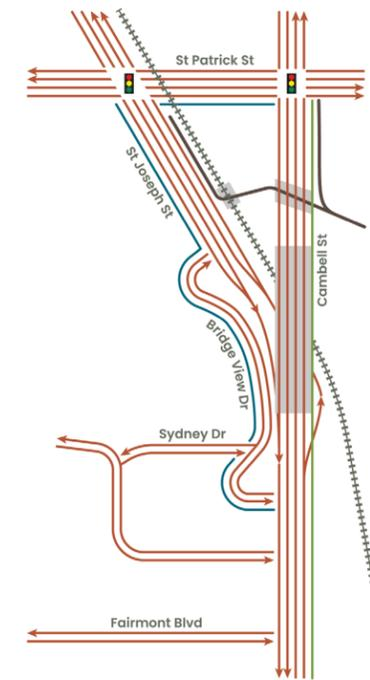
This alternative would adjust the alignment of St. Joseph Street to cross the railroad (at-grade or via a structure) and intersect with Cambell Street at a 90-degree angle south of the existing warehouse facility at 1313 St. Patrick Street. A traffic signal would be installed at the new intersection of St. Joseph Street and Cambell Street, with sidewalks added to Cambell Street and St. Joseph Street.
